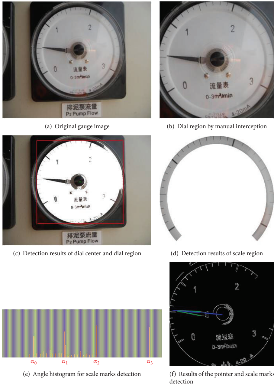
FIGURE 15: The detection results of the pointer gauge with an uneven scale.
